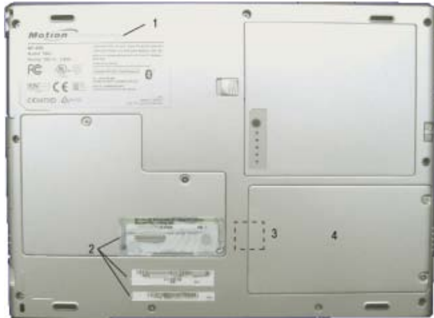
Motion Tablet PC Label Locations: (1) System Label; (2) Product Identification; (3) Internal Modem with label; (4) Hard Disk Drive Cover (remove to access modem)
